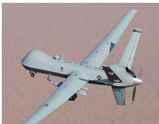
MQ-9 Reaper unmanned aerial vehicle equipped with AI-assisted systems for surveillance and target analysis. The expanding use of AI across military operations—from reconnaissance to targeting and decision support—raises growing concerns about accountability, escalation risks, and the potential normalization of autonomous or semi-autonomous lethal force. Photo by Lt. Col. Leslie Pratt (Wikimedia Commons).
